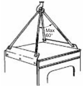
When hoisting with a crane, the lifting plate attachments should be mounted on the cubicles.
