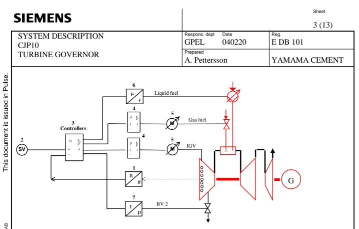
The actual values of the speeds are brought to the governor as a pulse train. Other feedback is transmitted in the form of standard current signals. In the various control channels the actual values are compared with their respective set values. The difference between actual and set value gives an error signal that then, properly manipulated, form the governor output signal. The output signal is proportional to a valve position or a liquid fuel pump speed respectively.
