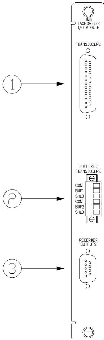
1) Connect the I/O module to the External Termination Block using cable 135101-XXXX-XX.
