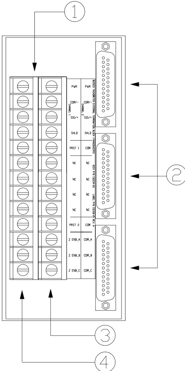
1) Connect the wires from the transducers associated with Channels 1 and 2 to the External Termination Block.
