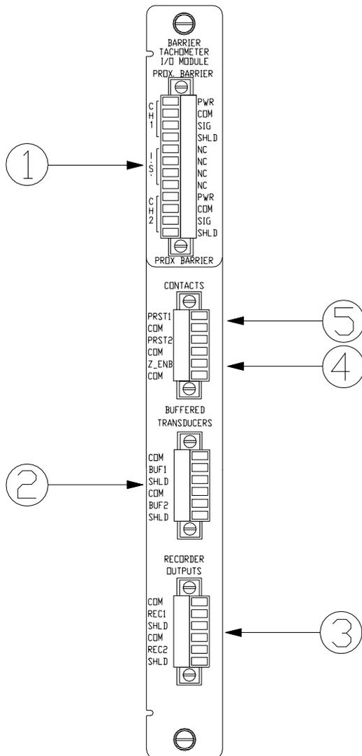
1) Connect the wires from the transducers associated with Channels 1 and 2 of the Tachometer Internal Barrier I/O Module.
