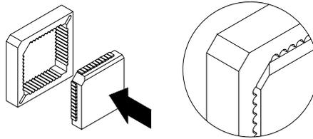
Install the upgrade firmware IC into the PWA. Be sure that the keyed corner on the IC is matched to the keyed corner of the socket. Ensure that the IC is firmly seated in the socket.
