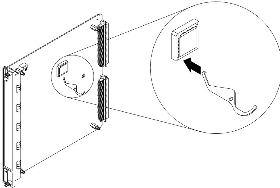
Step 1. Insert the removal tool in one of the two slots at the corner of the socket on the PWA. The diagram shows the approximate location of the chip to be removed, but not necessarily its orientation.
