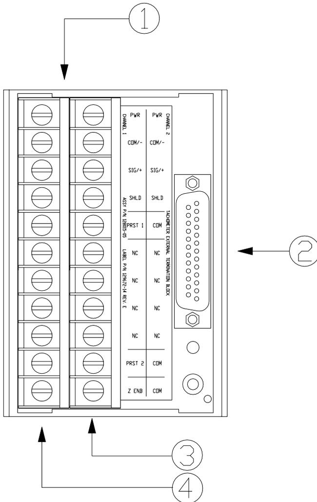
1) Connect the wires from the transducers associated with Channels 1 and 2 to the External Termination Block
