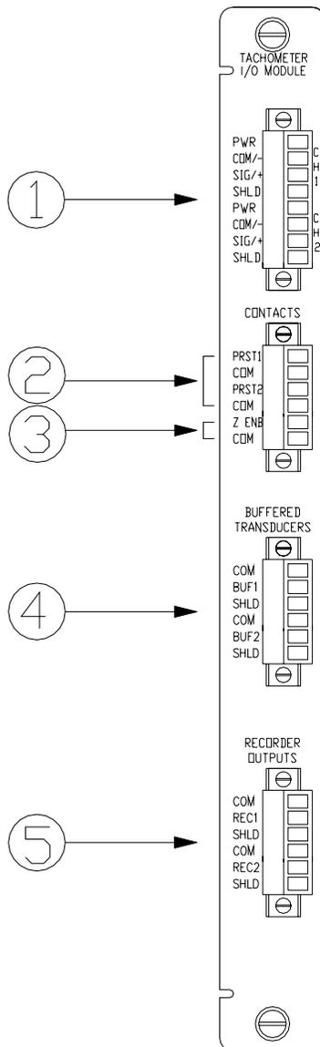
1) Connect the wires from the transducers associated with Channels 1 and 2 of the Tachometer I/O Module.
