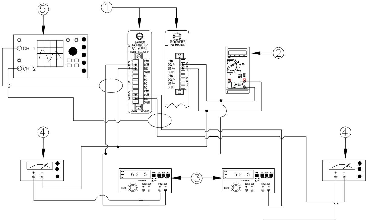
**Figure 5-1. Tachometer Test Setup**
