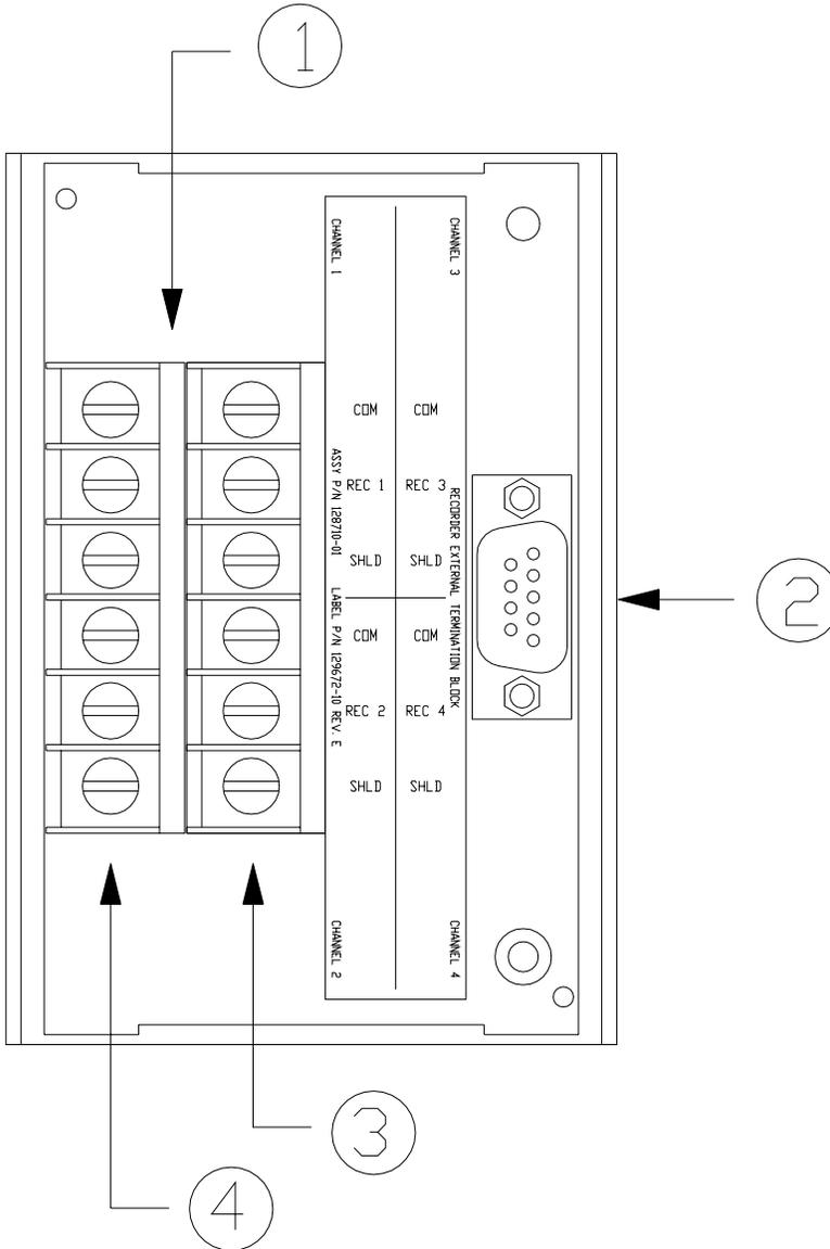
1) Connect the recorders associated with Channel 1 and 2 to the Recorder External Termination Block.
