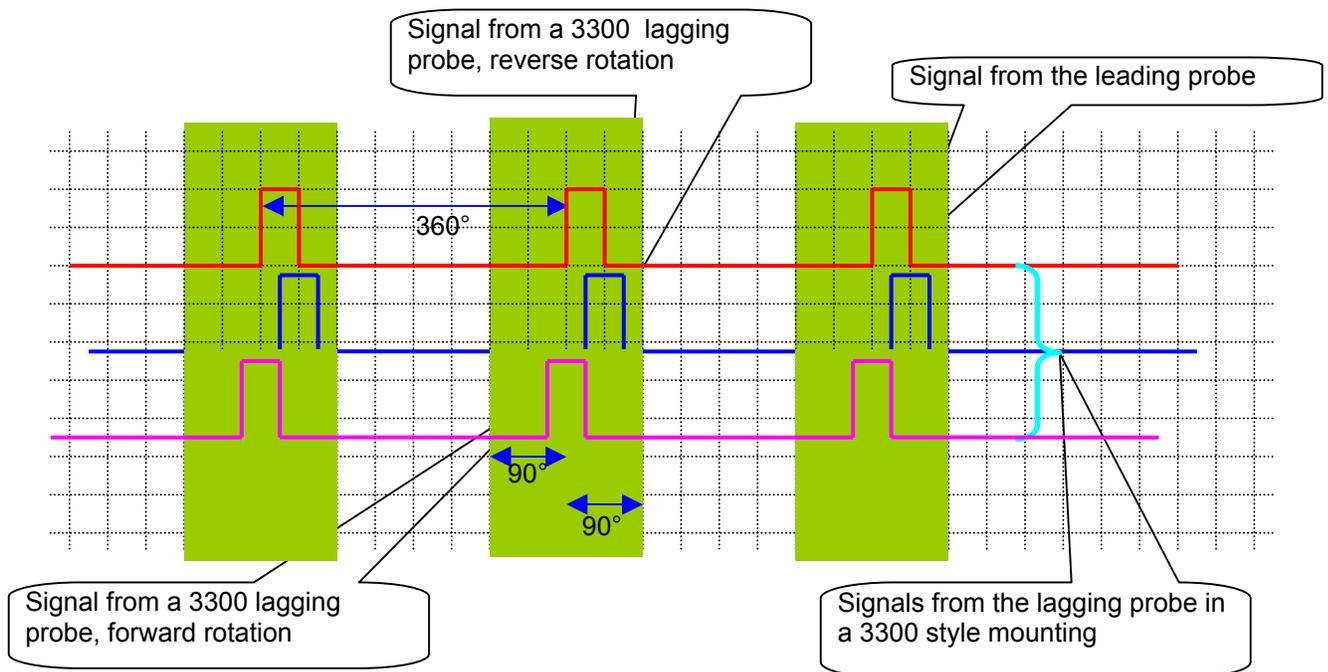
If the signal from the leading probe is as shown in the figure, then the rising edge of the lagging probe must fall in the shaded region to properly detect a reverse rotation condition. The signals from a 3300/52-style probe mounting meet the requirements of a 3500 reverse rotation channel type and thus the 3500/50 reverse rotation channel type supports 3300/52 style mounting.
